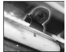
P-Clip keeps cord in-place (prevents cord damage).
