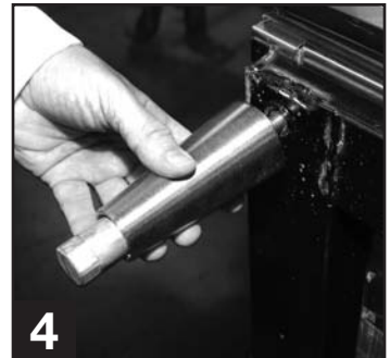
4 Thread leg into cabinet bottom frame rail.
