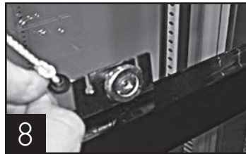
Door roller bracket with nylon cord.
